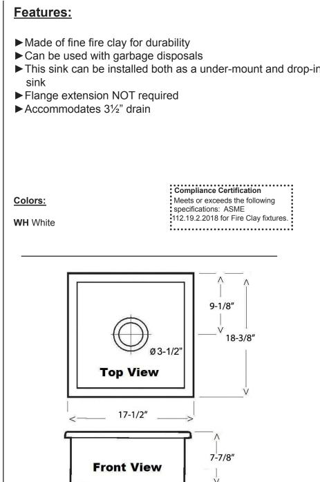
Dimensions of fixture are nominal and may vary within the range of tolerances established by ANSI Standard A112.19.9. Dimensions and specifications subject to change without notice.
